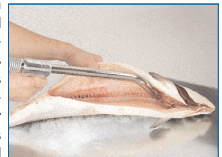
Model LKE-1 Vacuum Gun for removing salmon kidneys and bloodlines.
