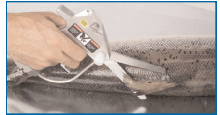
Model 35PA-2 Airsnip® is ideally suited for removing fins, heads and tails.
